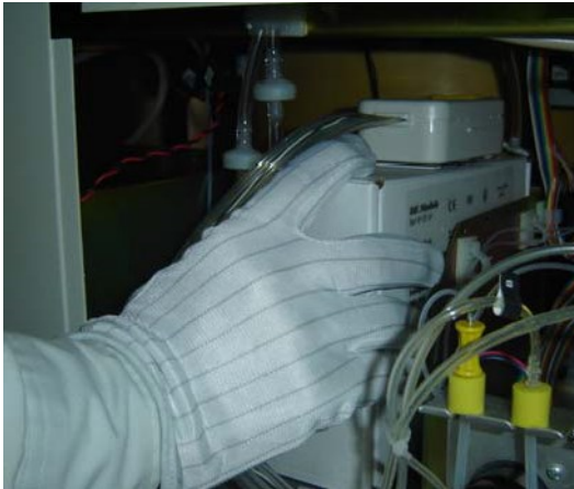
Figure 2-7 Install Reagent Pack Step 3
