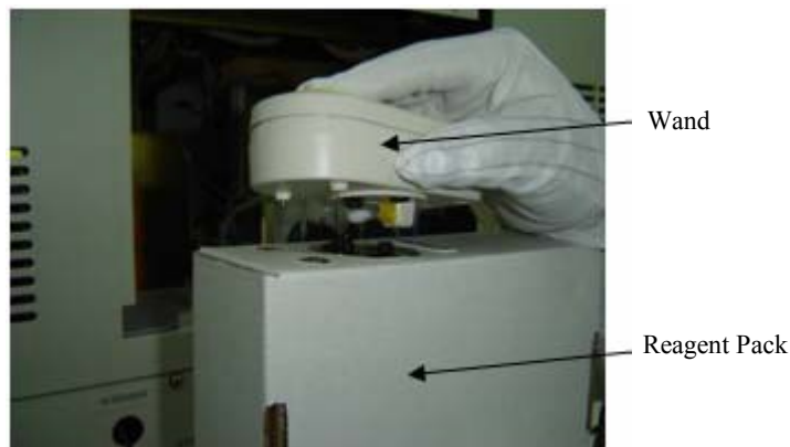
Figure 2-5 Install Reagent Pack Step 1
