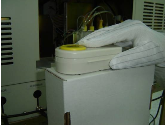
Figure 2-6 Install Reagent Pack Step 2
