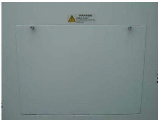
Figure 2-4 Remove back cover of analyzer
