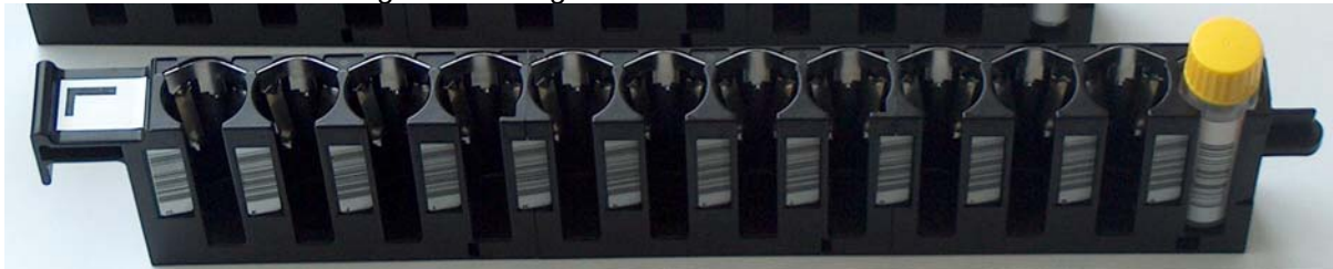
Fig 13.2.4-1: Light Check inserted in an rack
