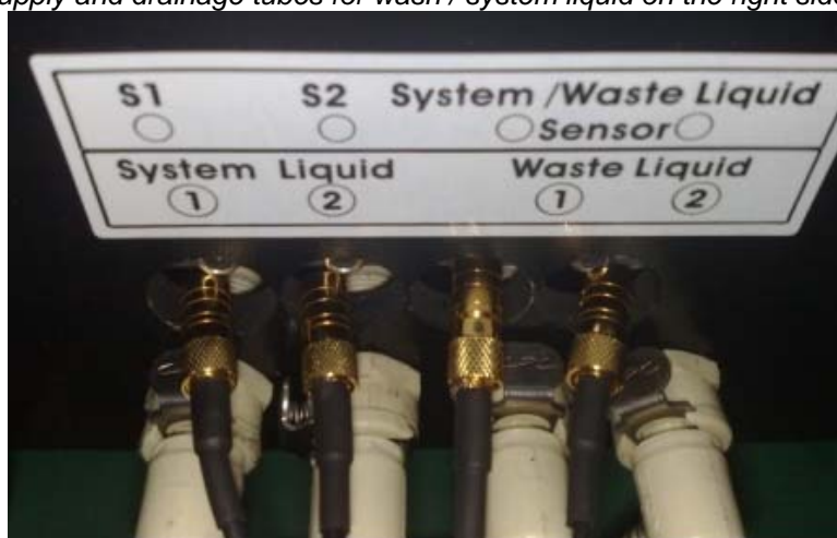
Fig. 3.2.11-1: Supply and drainage tubes for wash / system liquid on the right side of the analyzer.
