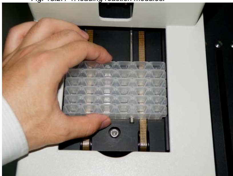
Fig. 13.2.1-1: loading reaction modules.
