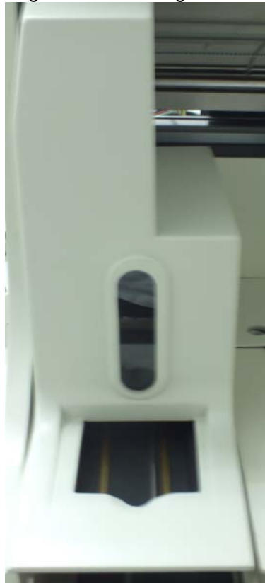
Fig. 3.2.9-1: Loading with reaction modules.
