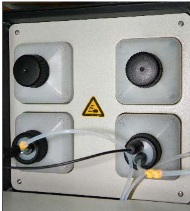
Fig. 9.3-1: Warning Label on Starter Reagent container on the right side of the analyzer
