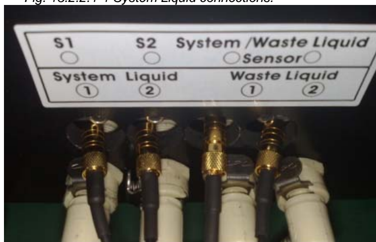
Fig. 13.2.2.1-1 System Liquid connections.
