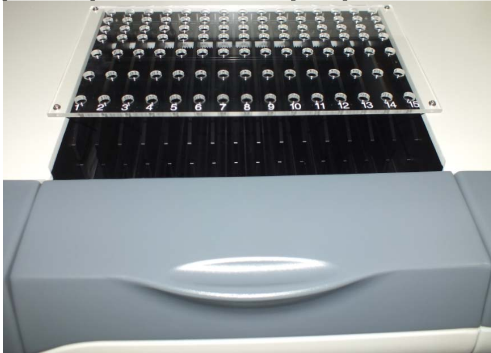
Fig. 3.2.2-2: Reagent station with 15 tracks for Reagent Integrals MAGLUMI 1000/2000.
