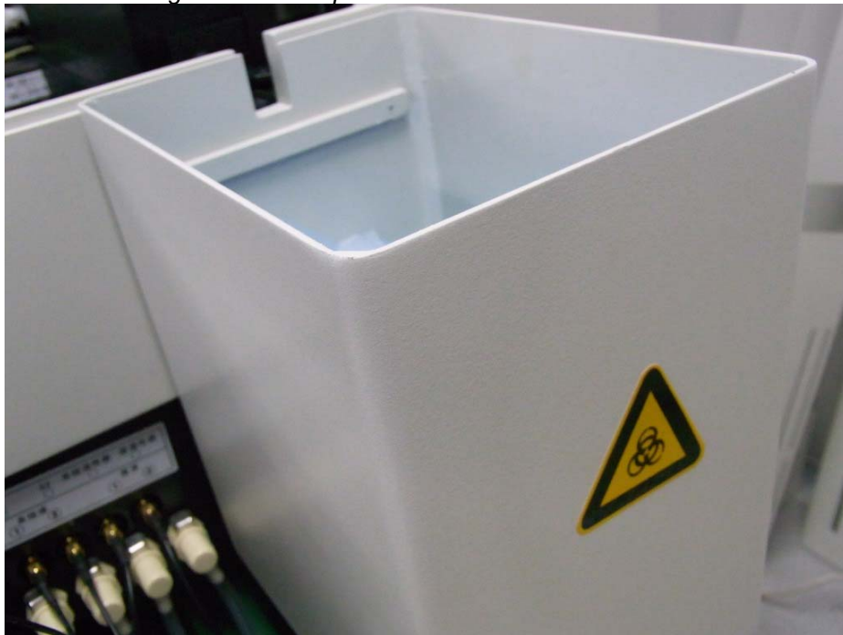
Fig. 3.2.12-1: Disposal of reaction modules
