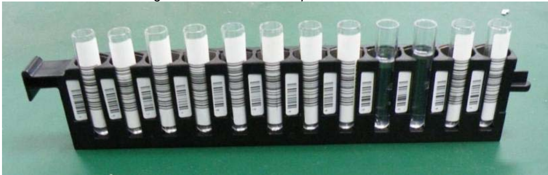
Fig 15.2.2-1 Bar-code sample tubes in a rack
