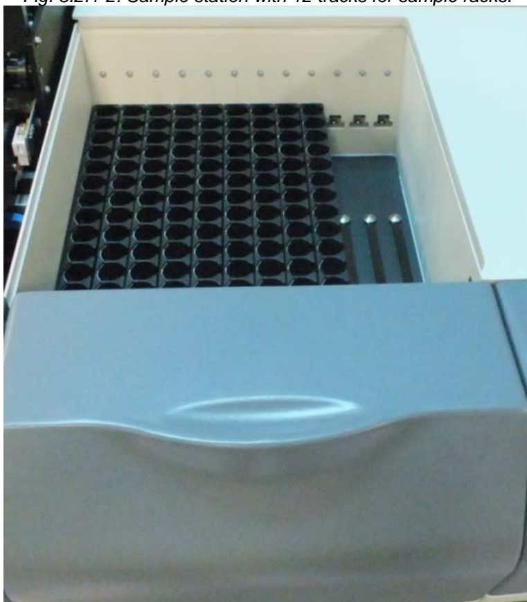
Fig. 3.2.1-2: Sample station with 12 tracks for sample racks.
