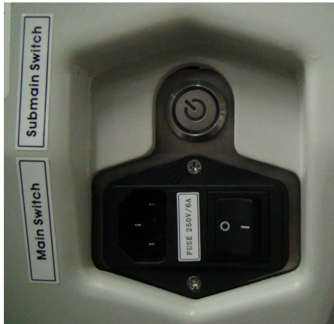
Fig. 3.2.12-1: Electrical and electronic connections.
